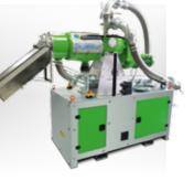
SEPARATOR Press screw separator for solid-liquid separation
