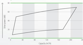
Tractor gear pump with 540 rpm. All values apply to water.
